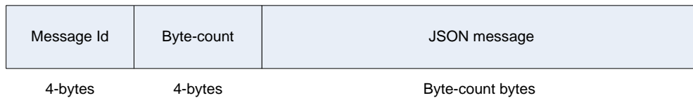
Figure 15 - Message format over the TCP channel
